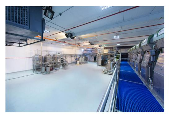
the contractor surface-prepped the entire cooler floor by grinding and shot-blasting, preparing it for the contoured floor that required up to 3-inches of epoxy mortar. Crews sloped the final surface from the outside walls to new trench drains.
